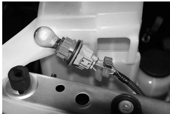
Figure 9 - Turn Signal Wiring Access
