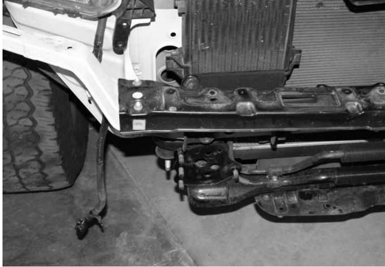
Figure 3 - Factory Bumper Connection
